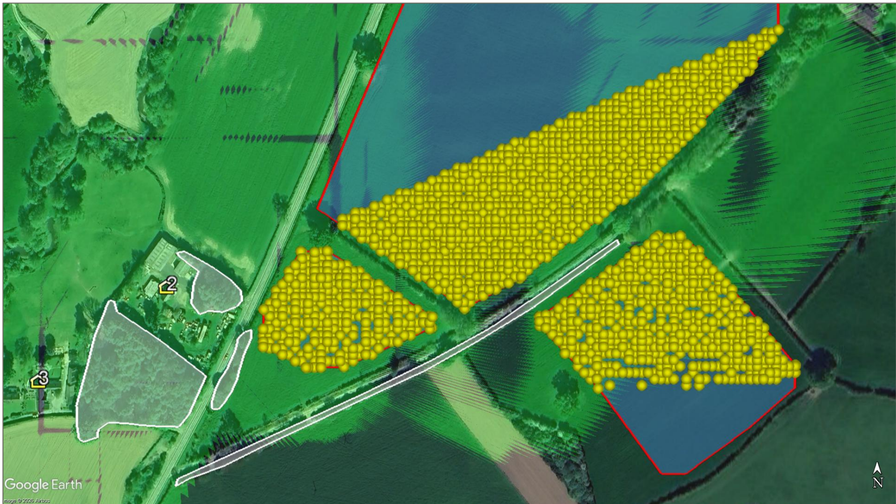
Figure 10 Screening relevant to dwelling receptors 2 and 3, with ZTV viewshed showing representative terrain visibility from dwelling 2
